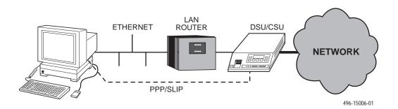
Figure 2-4. Direct Connection
